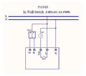
Fig 1. PAN03 Assembling
